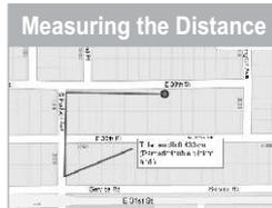
The travelled distance can be measured on the Map. Click "Measure", then click the position that will be measured on the map, double-click to end.
