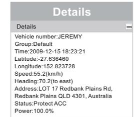
This column shows vehicle's license plate number, group, time of record uploaded, Longitude, latitude, Speed, Direction, Address, status, Signal of GPS and GSM, Battery Volume.
