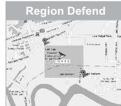
Under the region defend, an area selection window will pop out, click on the area button above the map, and point the cursor on two positions and click out an rectangular region, then confirm the drawn region by click on set tab to complete the geo-fencing process.
