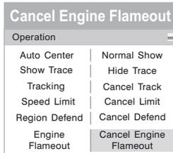
Click "Cancel Engine Flameout" to pop up the settings interface, input the password of device and confirm this operation. About 1 minute after apply the setting; the "Engine Flameout" signal will be cancelled.
