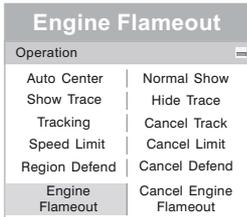
Click "Engine Flameout" to pop up the settings interface. After entering password and confirming, click the Enable key to start the remote flameout for the vehicles. About 1 minute after apply the setting, information bar will show "Engine Flameout" to signal.
