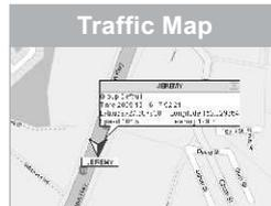
The blue icon in the Google traffic map shows the vehicle's location. When device has not uploaded positioning data in 10 minutes, icon will turn grey. When device uploads alarm information, icon will turn red. When replaying the historic trace, icon will turn green.
