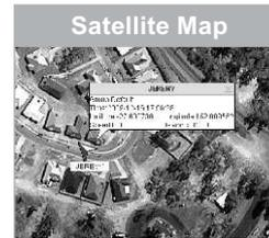
The blue icon in the Google satellite map shows the vehicle's location. When device has not uploaded positioning data in 10 minutes, icon will turn grey. When device uploads alarm information, icon will turn red. When replaying the historic trace, icon will turn green.
